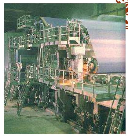
In the main elements (preparing the fibres, dewatering with a filter, pressing, drying) the production of paper is still the same as at the beginning
